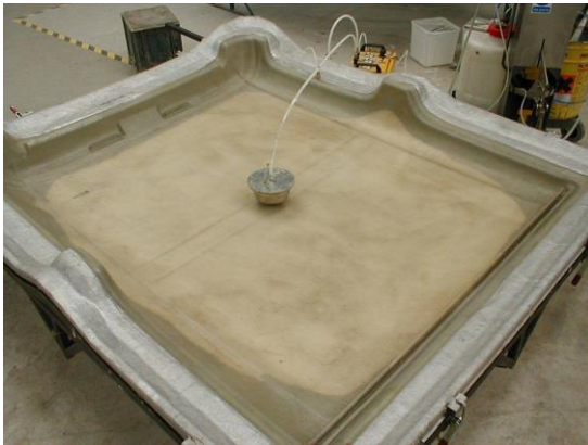
A moulding being filled peripherally
